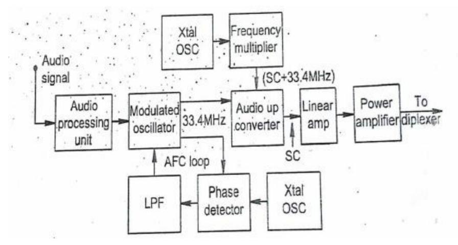
Using the linear and power amplifier the audio signal is amplified to the required level and is fed into the diplexer unit along with the video signal.
