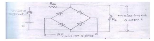
A bridge diode modulator or a diode balanced modulator is used for LLM.
