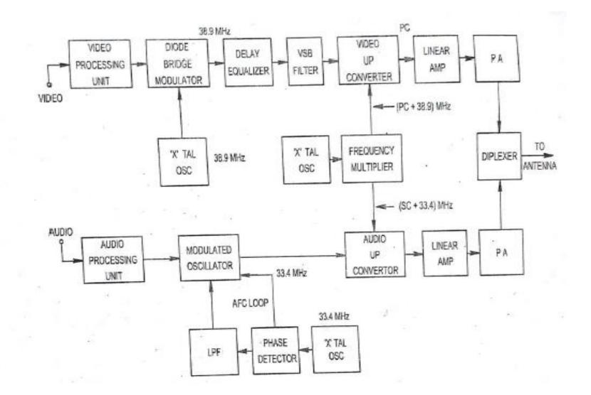
In this video modulation is done at IF frequency of 38.9 MHZ and sound modulation is done at IF frequency of 33.4 MHZ. Both video and sound IF UP converted after modulation. A VSB filter is also included at lower IF power level. After up conversion they are given to lines, amplifier for power amplification and then it is connected to the diplexer unit.
